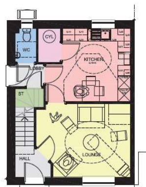
GROUND FLOOR LAYOUT HOUSE TYPE B 2 BED / 3 PERSON HOUSE Ground Floor Area = 39,2m 2 Total Gross Internal Floor Area = 78,4m 2
